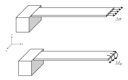
Applying the Stoney equation assumption that the surface stress bends the plate with uniform curvature, into the concentrated moment induced plate bending the following curvature relation for plate bending can be given as:
