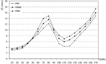
Figure 3. Impedance vs frequency at the CENELEC band for urban power lines [7].
