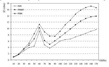
**Figure 4**. Impedance vs frequency at the CENELEC band for industrial power lines [7].
