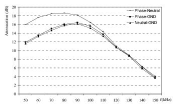
Figure 8. Power line attenuations for different locations the urban area.
