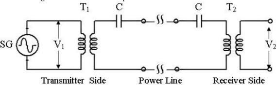
Figure 6. Test circuit of the power line attenuation measurements.
