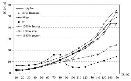
**Figure 5**. The effects of some house appliances on the impedance.
