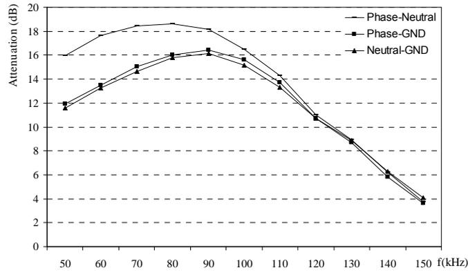
Figure 8. Power line attenuations for different locations the urban area.
