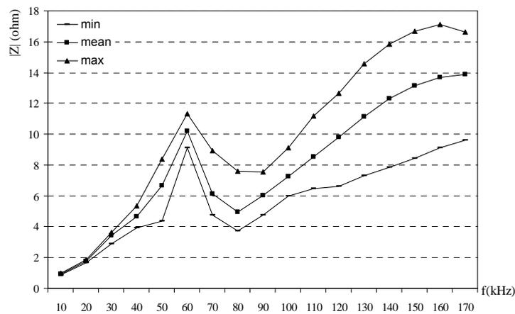
**Figure 4.** Impedance vs frequency at the CENELEC band for industrial power lines [7].
