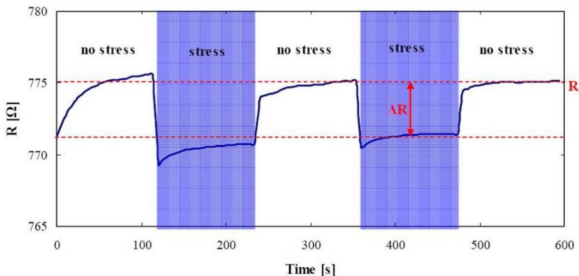
**Figure 12.** The two-point resistance,  $R$ , of a polyaniline thin film as a function of time. The colour correspond to periods where 160 MPa tensile stress is applied and the non-coloured areas correspond to periods without stress applied.
