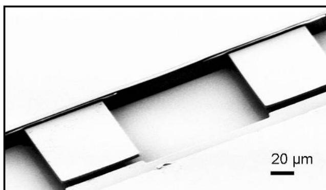
**Figure 6.** SEM image of two free-hanging cantilevers in the microfluidic channel. The cantilevers are 75  $\mu\text{m}$  wide, 100  $\mu\text{m}$  long and 4.5  $\mu\text{m}$  thick.
