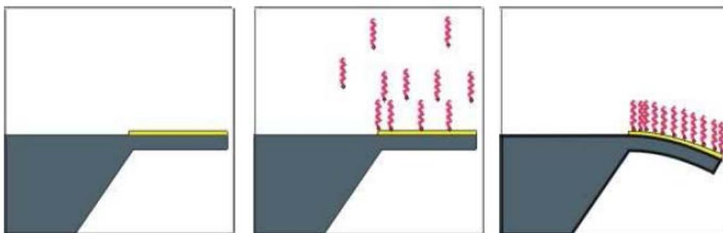
**Figure 1.** As molecules selectively bind to one surface of the cantilever, the structure is deflected due to the generated surface stress. Image courtesy Rodolphe Marie.
