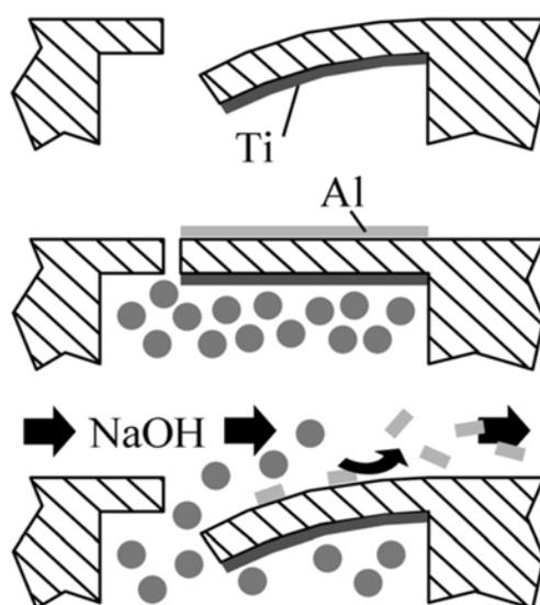
**Figure 13.** Here an Al layer is etched using NaOH to show the principle of operation of the micro valve. As the flapper is deflected the marker solution (filled circles) is released into the reacting liquid above.
