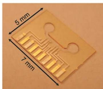
**Figure 9(b).** Optical image of the complete SU-8 chip. The cantilevers are situated in the micro channel. The Au contact pads are visible.
