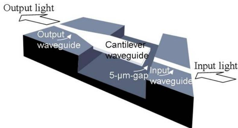
**Figure 7.** The light travels through the system, via the cantilever that also acts as a waveguide and is collected on the opposite side.
