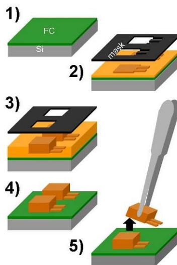
**Figure 2.** Schematic drawing of the different steps involved in the fabrication of the SU-8 cantilevers.
