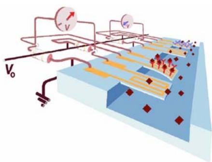
**Figure 9(a).** Schematic drawing of the four cantilevers with the integrated piezoresistors, situated in the micro channel.
