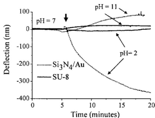
**Figure 5(b).** Compared to the Au coated  $\text{Si}_3\text{N}_4$  cantilever the fluorocarbon-coated SU-8 cantilever is less sensitive to pH changes [31].
