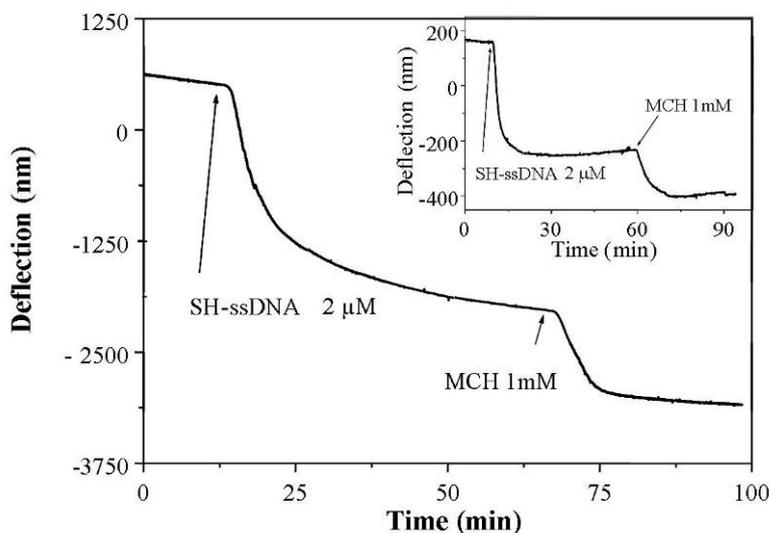
**Figure 4.** The introduction of 2  $\mu\text{M}$  ssDNA results in a six times larger deflection of the SU-8 cantilever (2500 nm deflection) compared to the  $\text{Si}_3\text{N}_4$  cantilever (400 nm deflection seen in inset) due to the lower Young's modulus of the polymer cantilever [31]. Both cantilevers are coated with a 20 nm thin layer of Au and the deflections are read out by the optical lever principle.
