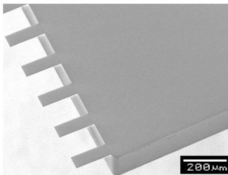
**Figure 3.** SEM image showing a 2- $\mu\text{m}$ -thin and perfectly straight cantilever. The width and length of the cantilever is 75  $\mu\text{m}$  and 200  $\mu\text{m}$  respectively.
