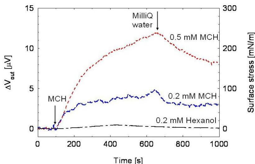
**Figure 10.** Surface stress measurements of chemisorptions of MCH on Au-coated SU-8 cantilevers.
