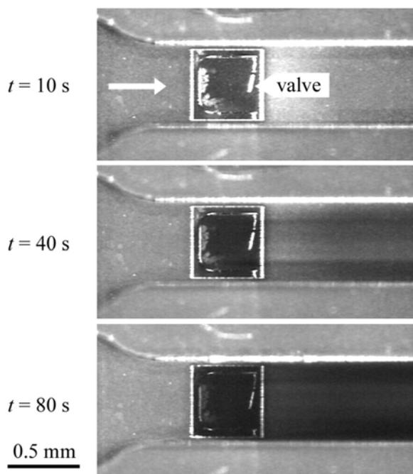
**Figure 14.** Optical microscope images showing the release of the marker solution from the lower reservoir into the reacting liquid flow channel as the Al layer is etched away by a 0.5 M NaOH solution. The arrow at the top indicates the flow direction.
