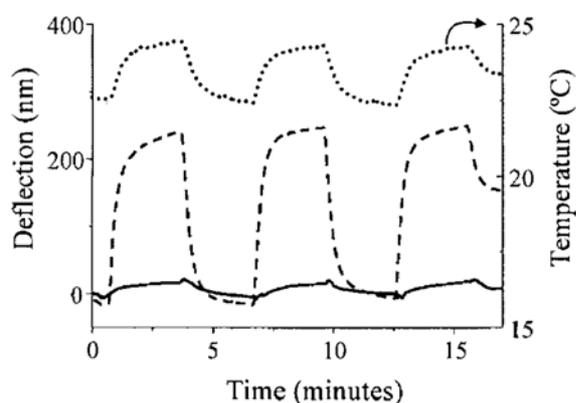
**Figure 5(a).** As the temperature is cycled between 22 and 24  $^{\circ}\text{C}$  the deflections of the  $\text{Si}_3\text{N}_4$  cantilever (dashed line) is 14 times greater than the deflections of the SU-8 cantilever (solid line). The reason for the difference is that the  $\text{Si}_3\text{N}_4$  cantilever needs to be coated with an Au layer for the immobilisation of molecules, something which can be done directly on the SU-8 surface [31].
