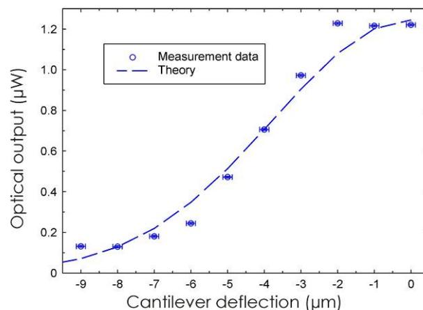
**Figure 8.** Comparison between calculated and measured values of the sensitivity. When operated in the most sensitive region, at an initial cantilever deflection of  $4$   $\mu\text{m}$ , a deflection resolution of  $45$  nm can be obtained.
