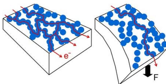
**Figure 11.** As the cantilever is strained, contact is broken between the conducting particles in the polymer and the resistance of the conductor is thereby increased.
