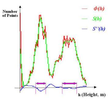
As presented in figure 2., to reduce the influence of slight amplitude movements on the function,  $\phi(h)$  is firstly smoothed with a gaussian function, a smoothed function S(h) is generated, the second derivative S''(h) is then calculated for the smoothed function S(h).
