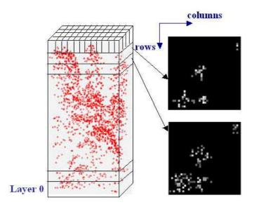
To simplify the computational complexity, a series of 2D horizontal projection images are introduced into the further analyses as an instrument to record the voxel space. Taking all the voxels of a single layer out of the voxel space, the voxels of the layer can be regarded as pixels of an image. The number of normalized points within each voxel is marked as a gray value of the correspondent pixel in the image. A 2D horizontal projection image of the selected layer is then generated (Figure 7.).
