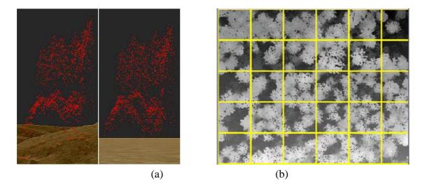
As shown in Figure 1.(a) Left, raw points are projected above the DTM, the height difference between a raw point and its correspondent terrain is marked as the normalized height of the point. A normalized point cloud is then generated (Figure 1. (a) Right), where point heights of the normalized point cloud represent the absolute heights of the objects.
