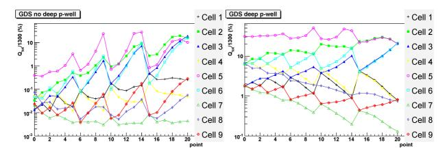
**Figure 9.** Simulation of charge collection for the (GDS) pixel layout data and an ideal (perfect) pixel containing only the collection diodes, as a function of the impact point and for the nine cells in the layout. On the left: with a perfect P-well. On the right: reference plot from Figure 8: standard pixel with deep P-well.
