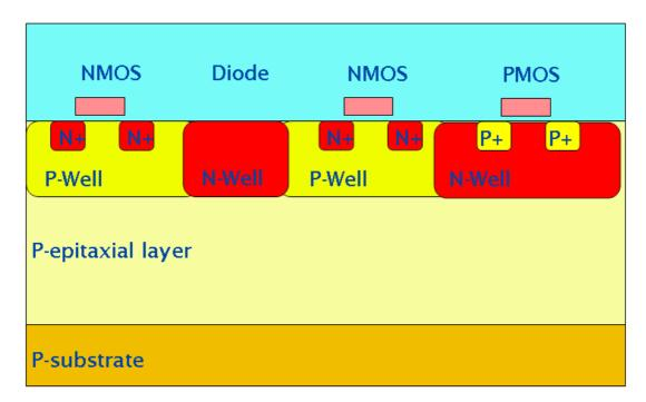
Figure 1. Schematic cross-section of a typical CMOS wafer. Not drawn to scale.
