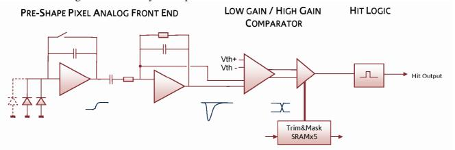
**Figure 4.** *PreSample* pixel block diagram showing the analogue signal path from collecting diodes to binary *hit* output.
