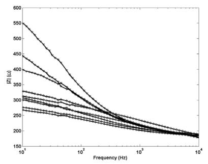
A selection of electrochemical impedance data for the three structural Ag/AgCl designs is presented in Figure 7. As expected no change is observed in shape between the profiles for each Ag/AgCl structure indicating the same porous structure in each. Electrodes with cylindrical Ag/AgCl structures
