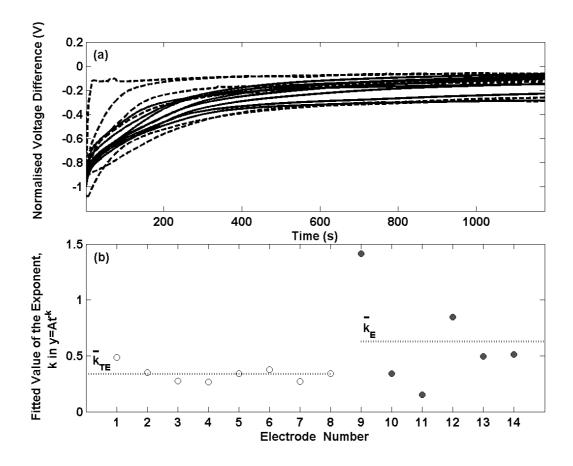
The porous structure of thermal electrolytic type limits the rate at which the electrodes can equilibrate, as any previous solution contained within the pores of the Ag/AgCl must diffuse out before
