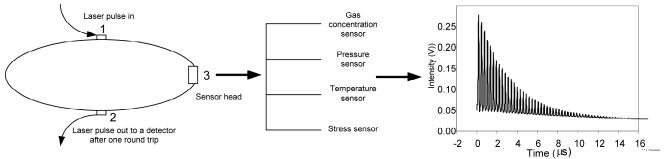
(a) Fiber loop ringdown sensing unit (b) Different sensor heads for different sensors (c) FLRD measures decay rates to determine a quantity
