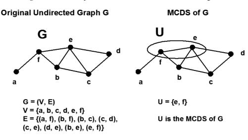
Figure 2. An example of Minimum Connected Dominating Set.
