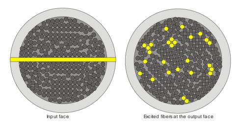
Sequential images are captured both in the horizontal and the vertical sweep. From these images it is possible to formulate a correspondence relationship between any excited input coordinate (i.e., row and column of a particular fringe), and any fiber location (previously determined) at the output face of the bundle which has been notably illuminated.
