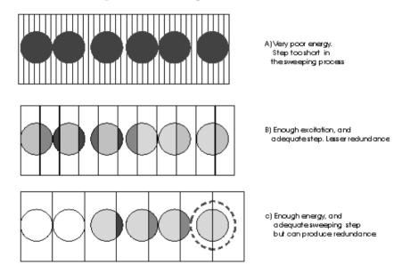
Figure 3. Scanning effect on the fibers.
