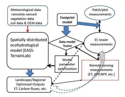
Figure 5 schematically shows a synthetic upscaling framework for estimating landscape and regional C and water budgets with a reasonable accuracy. Using a data-model fusion with footprint weighting method to optimize the ecohydrological model's parameters is strongly suggested because the land surface is normally heterogeneous. This is a key component in the upscaling framework. Model parameters are optimized by minimizing the 'cost' function [240]:
