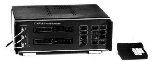
Figure 6. C-V, G-V meter for control of semiconductor characteristics.
