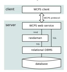
Figure 1. WCPS reference implementation service stack.
