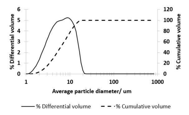
**Figure S2**. Coulter particle size distribution measurements for PS21 spray dried powder using inlet temperature 150°C. Differential volume distribution of particles (solid line), cumulative volume distribution (dashed line). Measurements were done in triplicate.
