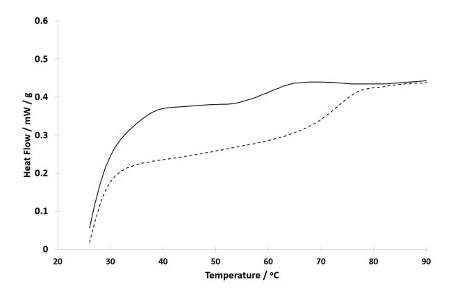
**Figure S4.** Differential Scanning Calorimetry of spray dried trehalose powders spray dried trehalose powders (PS04) showing the effect of spray drying inlet temperature 120 °C (solid line) and 150 °C (dashed line), on glass transition temperature.
