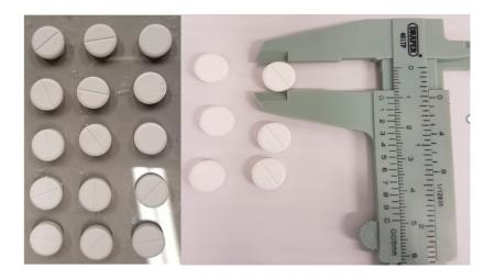
**Figure S3.** Images of tablets produced using the process of direct compression on spray dried powders PS21.
