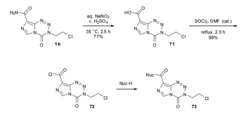
Scheme 22. General synthesis of esters and amides via MTZ acid chloride [78].
