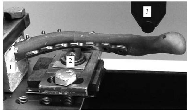
Fig. 1. The mechanical testing of the clavicle repaired by anteroinferior plating osteosynthesis
