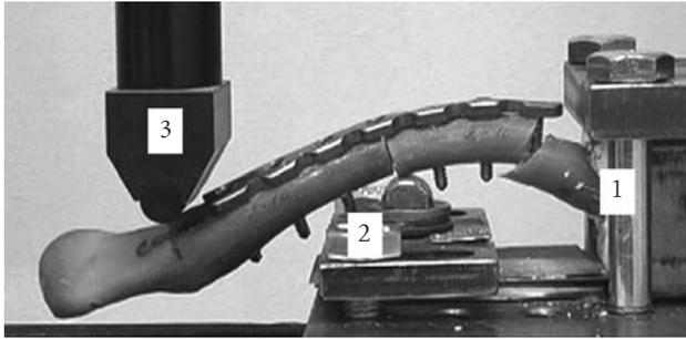
Fig. 3. The breakage of the repaired clavicle
