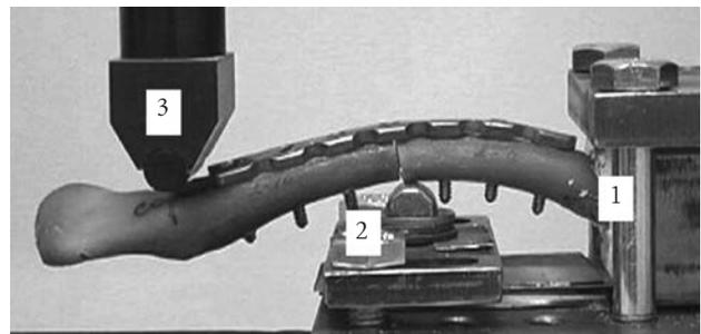
Fig. 2. The mechanical testing of the clavicle repaired by superior plating osteosynthesis
