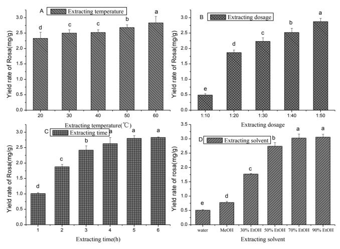
The L<sub>9</sub> ( $3^4$ ) orthogonal experiment was performed based on each parameter described above that affects extraction efficacy. The optimal conditions to increase RosA extraction is by using an extraction dosage at 1:50 and using 70% ethanol with an extraction time of 3 h at 40 °C (Table 3). A validation experiment was performed using these optimized conditions, and RosA was extracted at a concentration of 3.13 mg/g.
