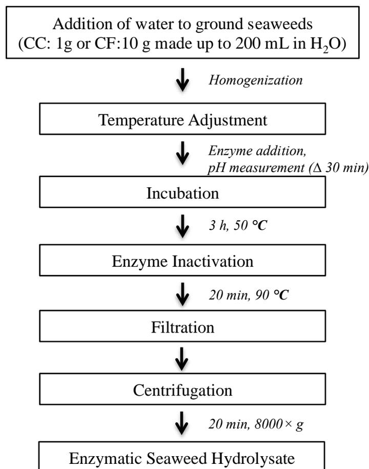
**Scheme 1.** Schematic representation of seaweed extraction process.
