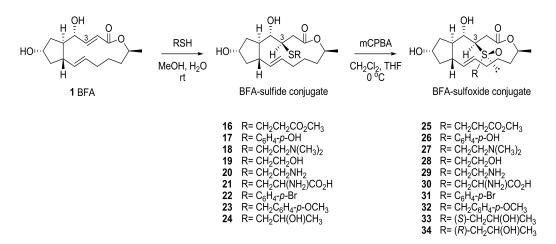
Scheme 6. Synthesis of sulfide- and sulfoxide-conjugated BFA analogs.
