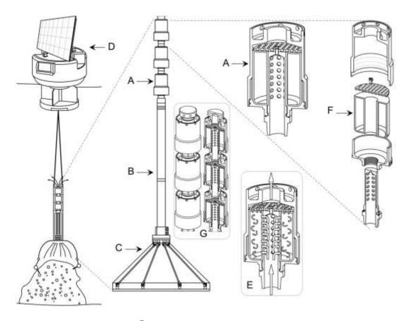
**Figure 6.** Drawing of Somartex<sup>®</sup>. **(A)** trapping module; **(B)** submersible pump; **(C)** cover dome; **(D)** Somartex platform; **(E)** water circulation inside the module. The water is forced to pass through the trapping material (ex. XAD resin) present in the **(F)** compartment, through the holed tube. The water can then reach the second module through the holed grid; **(G)** superposition of different modules that may contain different means of molecular trapping.
