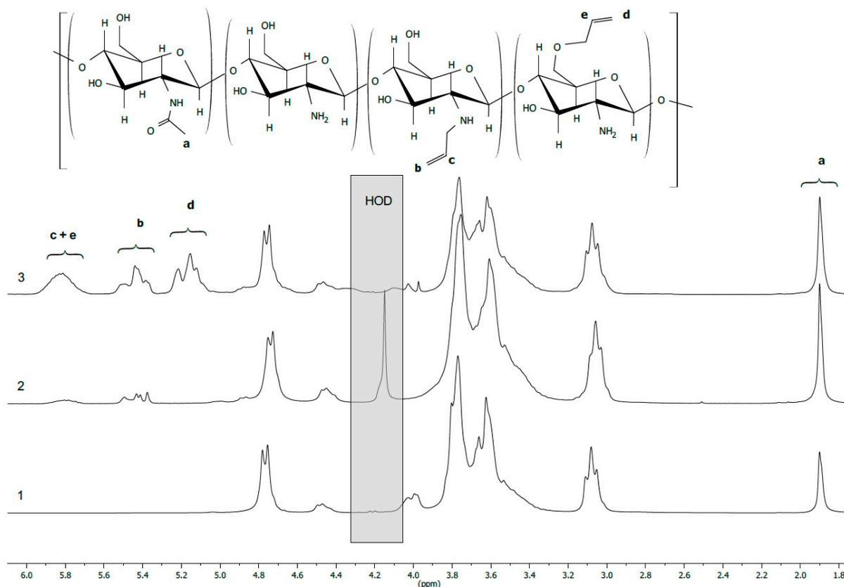
Figure S7. <sup>1</sup>H NMR spectra of chitosan (1), AC2 (2) and AC5 (3).
