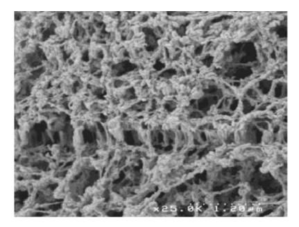
**Figure 4.** Removal of chitosan leads to pure titanium oxide with filamentous structure. Reprinted from [107]. Copyright (2011) with permission from Elsevier.
