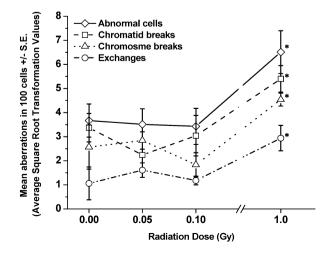
**Table 5.** Cytogenetic data from bone marrow cells collected at 1 mo after exposure of male SCID/J mice to varying low doses of  $^{137}$ Cs  $\gamma$  rays, including a high dose of 1.0 Gy serving as a reference dose. Both chromatid- and chromosome-type aberrations were detected.
