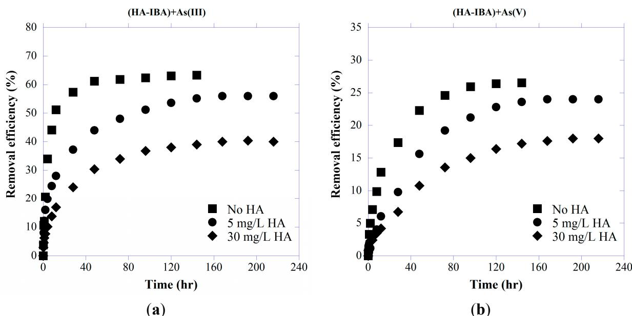
Although IBA preloaded with HA is net negative at pH 7.5, its small positive domains may be accessible, and contribute electrostatic attractions. It is thus assumed that adsorption in the studied pH
