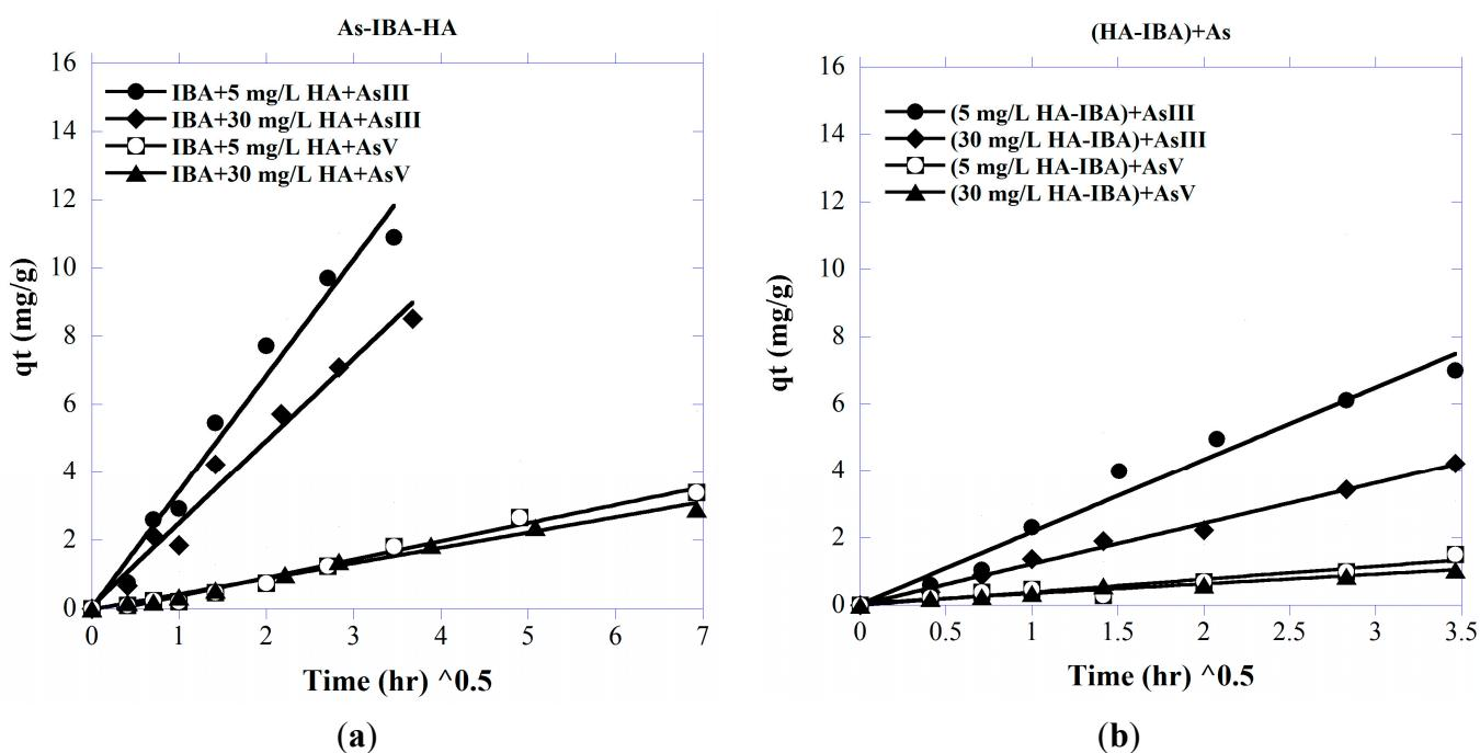
The values of  $k_{id}$  for HA preloaded systems indicate that the intraparticle diffusion rate for As species is higher at lower concentrations of HA. As pore dimensions decrease due to the adsorption of the competing HA, the free path for molecules to travel within the transport pores becomes smaller (with possible pore blockage occurring), and hence the transport rate decreases.
