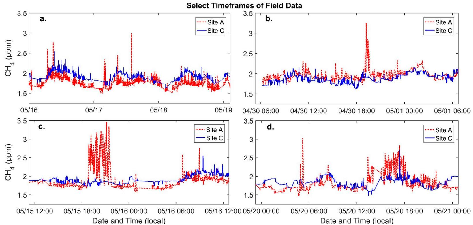
**Figure 3.** Select timeframes of field data that illustrate relatively large differences in methane between Sites A and C. (a) a period of four days including several examples of enhanced methane; (b) a 24-h period including an approximately 1 ppm increase in methane; (c) a 24-h period depicting an approximately three-hour long methane enhancement; (d) a 24-h period including several enhancements in methane.
