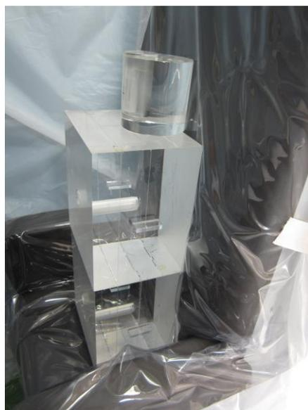
**Figure 2.** Thyroid phantom on the acrylic block phantoms.
