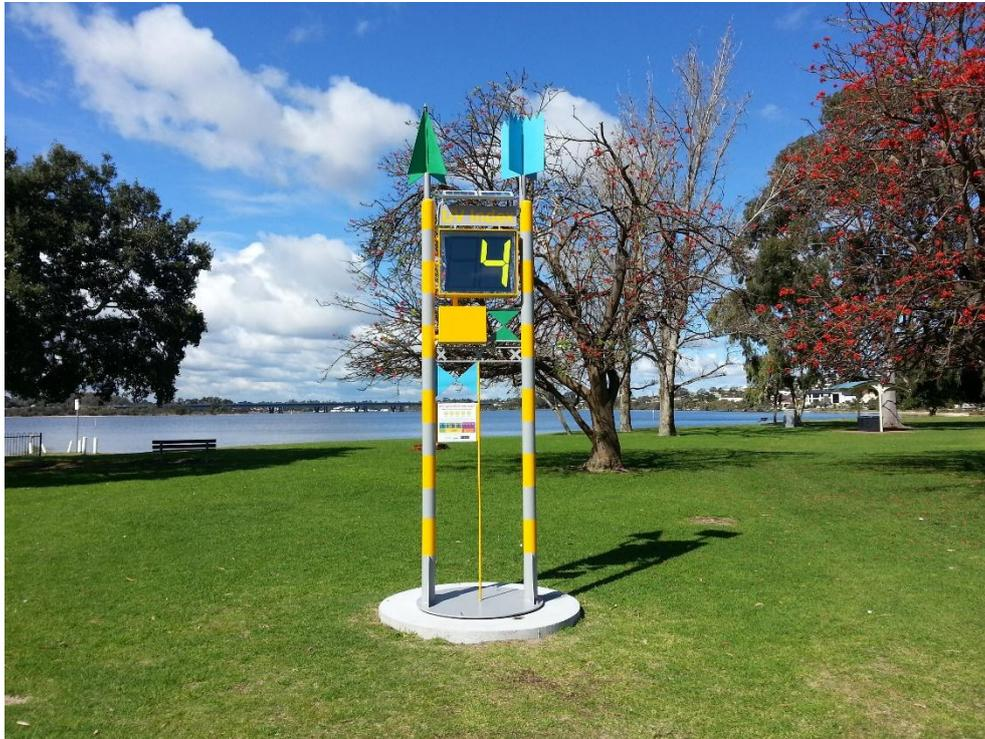
**Figure 4.** A UV meter displaying the live UV Index at Deep Water Point Reserve in Western Australia (Image courtesy of Cancer Council Western Australia).
