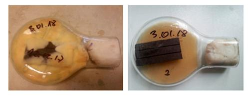
**Figure 2.** Kolle flask with *Coniophora puteana*—experimental chamber (on the left) and control chamber (on the right) after two weeks of incubation; photo taken by one of the contributing authors.
