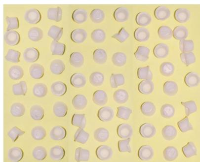
**Figure 5.** A total of 72 copings were milled according to test coping produced in order to evaluate the right fit.
