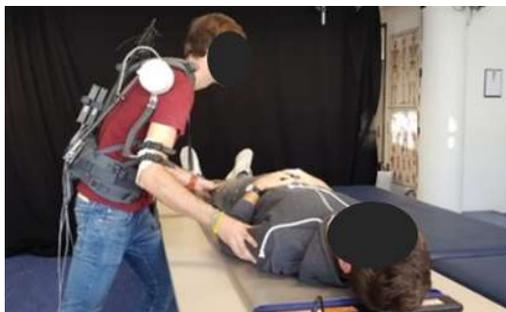
**Figure 18.** Preliminary laboratory tests with a prototype of the investigated exoskeleton design during the patient push scenario.
