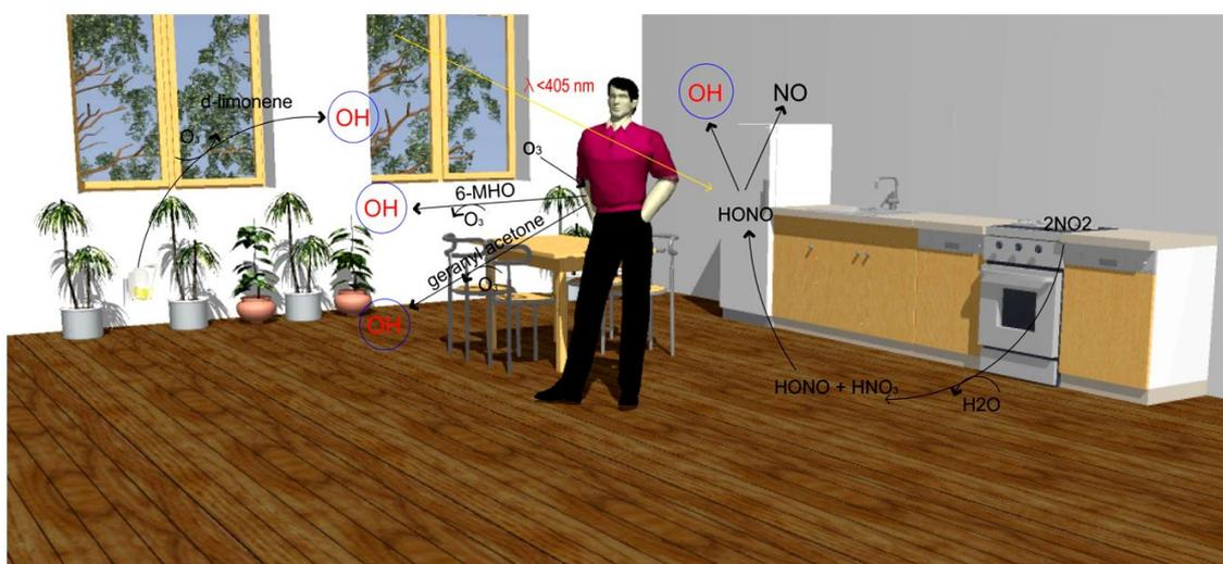
**Figure 1.** Schematic illustration of the important formation pathways of OH radicals indoors. Reproduced with permission from [118].
