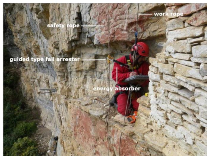
**Figure 14.** Archaeologist using a double rope. The line on the left is an energy absorber. La Joya site, Leymebamba, Amazonas Department, Peru.
