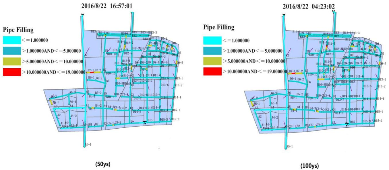
**Figure 9.** Simulation results of the influence of the designed rainfall process on the pipeline filling degree in the southern region under different design return periods (A1–D15 are the numbers of the pipes and nodes).
