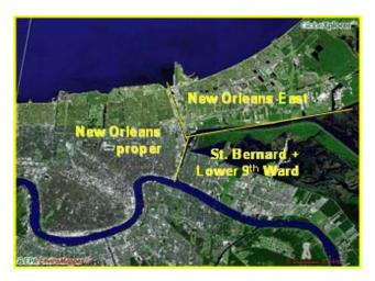
**Figure 2:** Map of New Orleans and neighboring areas showing the partitioning of the pump-out. Flood waters from New Orleans proper and New Orleans East were largely pumped into Lake Pontchartrain. Flood water from St. Bernard Parish and the Lower Ninth Ward of New Orleans were largely pumped into Violet Marsh.
