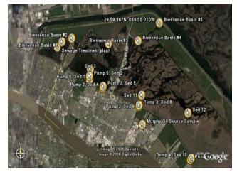
**Figure 3:** Map illustrating the sediment core locations with respect to the sewage treatment plant and stations that pumped flood water over the levee and into Violet Marsh. The GPS coordinates for the core locations are given in Table 1.
