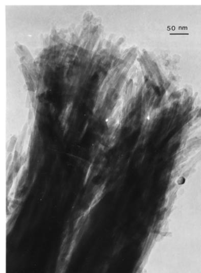
**Figure 15:** TEM image of MWCNT bundle collected indoors on an electrostatic plate.
