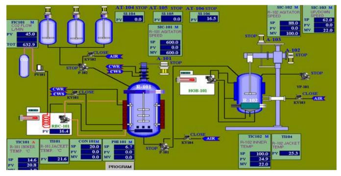
(a) Schematic of PCC process system
