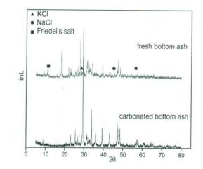
(b) Chloride removal by carbonation process: both soluble (KCl and NaCl) and insoluble (Friedel's salt) chloride were removed.
