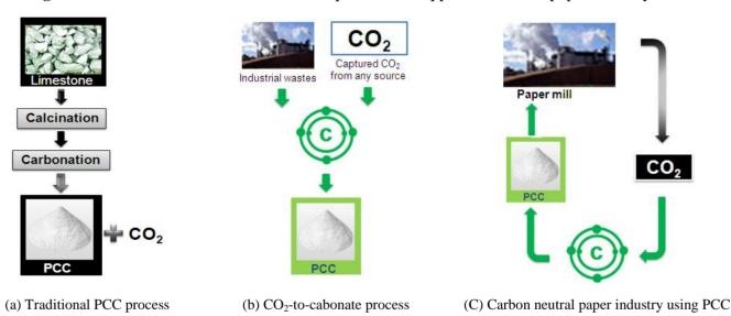
Figure 15. Schematic of PCC manufacture process and application to the paper industry.
