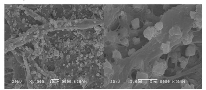
Figure 24 shows photos of the recycled papers made from three kinds of waste pulp through the *in-situ* process with PCC (10% calcite) in our laboratory, and the order of whiteness degree of the three recycled papers was as follows: (a) the recycled paper made from old newspaper < (b) the recycled paper made from white ledger < (c) the recycled paper made from printing paper.
