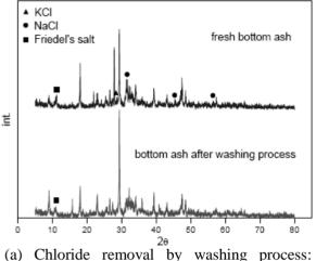
soluble chloride (KCl and NaCl) was removed but insoluble one (Friedel's salt) was not.
