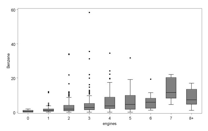
**Figure 2.** Benzene levels in ppb vs. total number of engines kept in the garage.
