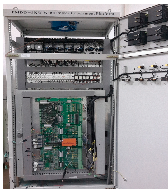
Figure 17. The experimental platform of stability analysis in inverter-grid system.
