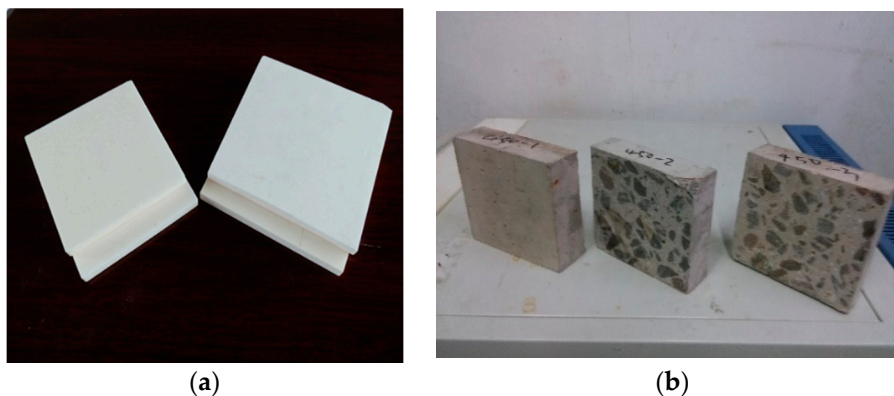
Figure 4. Test samples of corundum blocks and concrete blocks. (a) Corundum blocks; (b) Concrete blocks.
