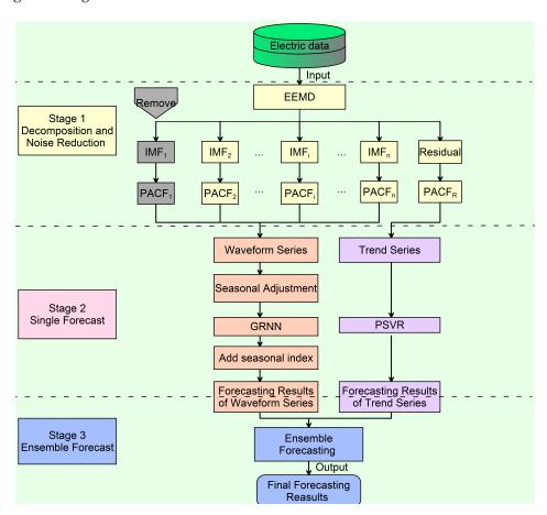
**Figure 3.** Overall flowchart of EEMD-SCGRNN-PSVR. EEMD: combines ensemble empirical mode decomposition; IMF: intrinsic mode function; PACF: partial auto correlation function; PSVR: support vector regression machine optimized by the particle swarm optimization algorithm.
