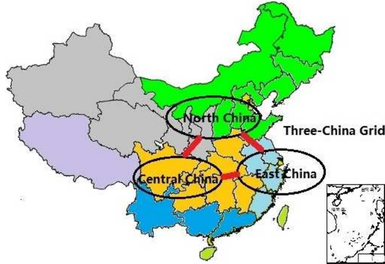
Figure 1. Diagram of the Three-China synchronous 1000 kV grid.
