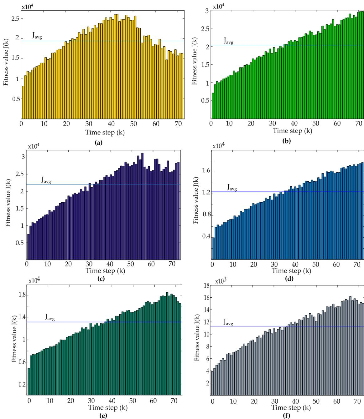
**Figure 3.** Cost function values  $J(k)$  obtained for a simulated PHEVs’ smart charging scenario consisting of 50 PHEVs, corresponding to: (a) PSO; (b) GSA; (c) SMS; (d) GA; (e) FA and (f) RCA. In each case, the average values  $J_{avg}$ , corresponding to the average of all  $J(k)$  values obtained during a single simulation, are indicated.
