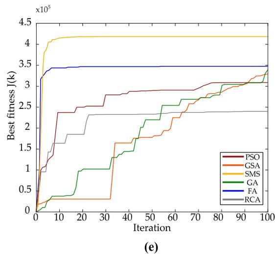
**Figure 4.** Evolution curves for PSO, GSA and SMS, considering several PHEVs' smart charging scenarios, consisting of (a) 50 PHEVs; (b) 100 PHEVs; (c) 300 PHEV; (d) 500 PHEVs; and (e) 1000 PHEVs.
