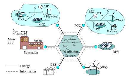
Figure 14. ADS architecture with multi-MGs.
