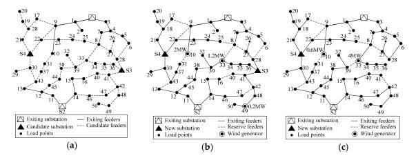
Figure 8. Case study based on 54-node distribution network (adapted from [89]). (a) Initial network;(b) Expanded network without active managements (AMs); (c) Expanded network with AMs.
