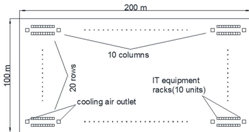
Figure 2. IT Equipment layout in the data center.
