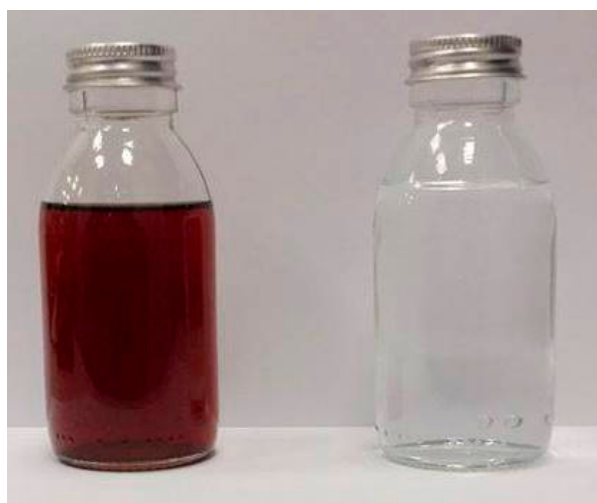
Figure 5. Mid-distillate fraction of waste plastics pyrolysis oil before (left) and after (right) catalytic hydrotreatment upgrading at CETH.
