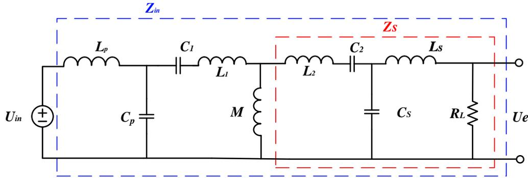
**Figure 2.** Equivalent schematic of double-sided LCC resonant compensation network.
