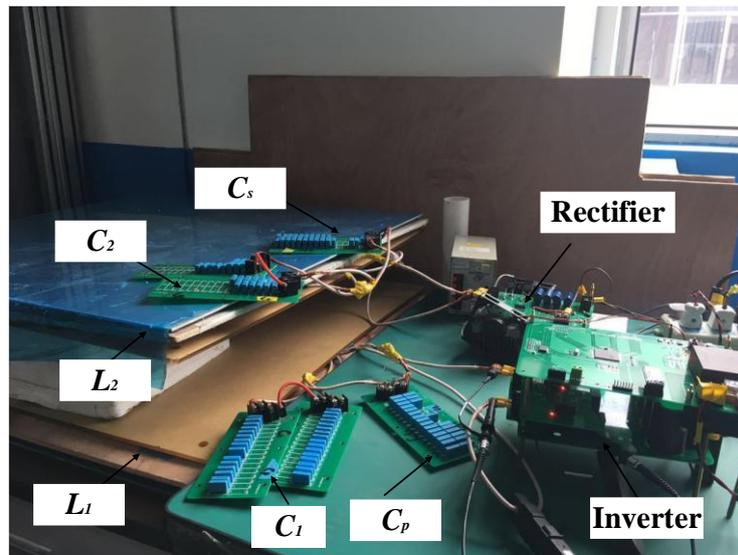
Figure 5. Experiment platform.
