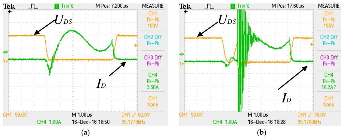
Figure 6. Voltage and current of MOSFET (a)  $t_{DT} = 500$  ns; (b)  $t_{DT} = 1.2$  us.
