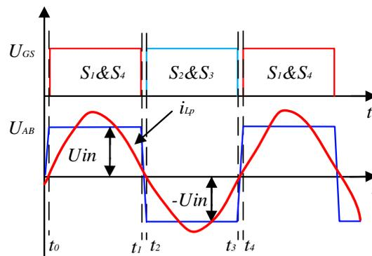
Figure 3. Operation waveform of the inverter.
