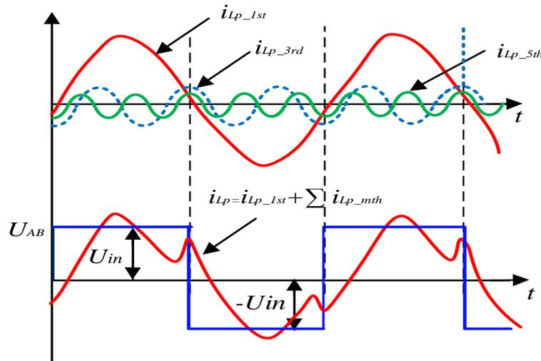
Figure 4. Effect of high order inverter current.
