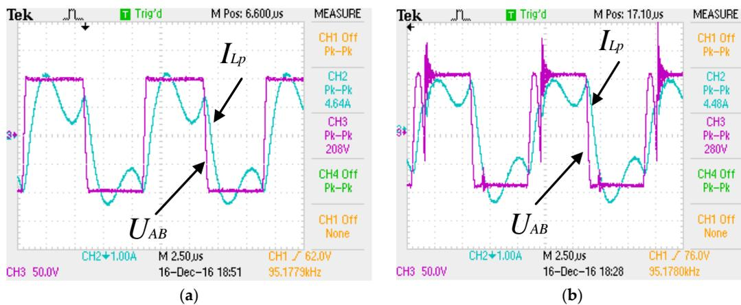
Figure 7. Voltage and current of inverter (a)  $t_{DT} = 500$  ns; (b)  $t_{DT} = 1.2$  us.
