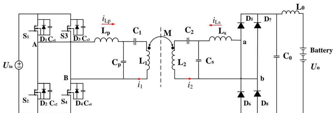
Figure 1. Schematic of double-sided LCC resonant compensation network.
