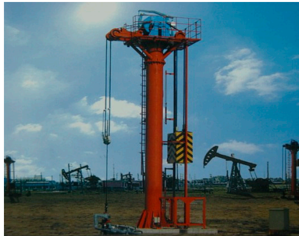
Figure 3. Compound permanent magnet synchronous motor pumping unit.
