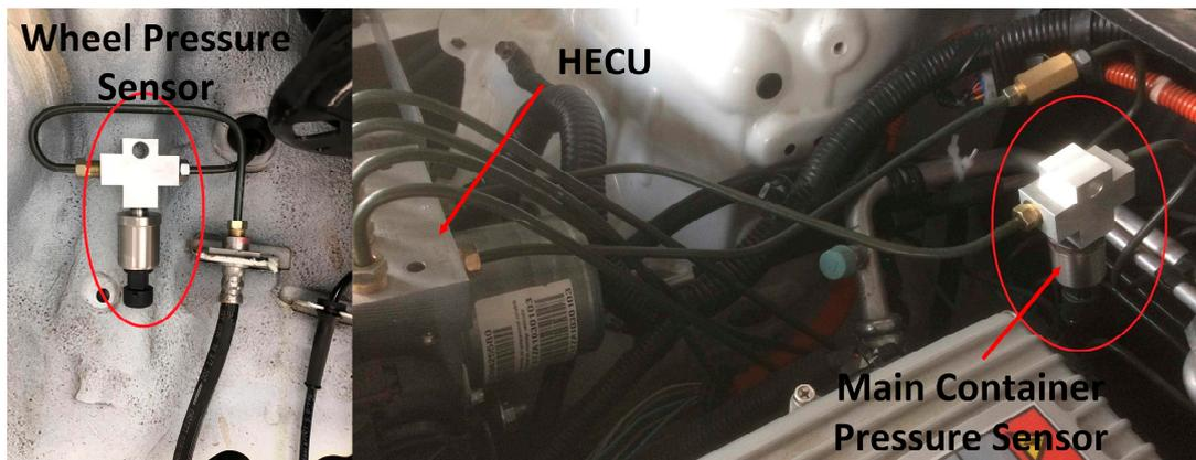
Figure 4. The pressure sensors mounted on each wheel and the main container pressure sensor.
