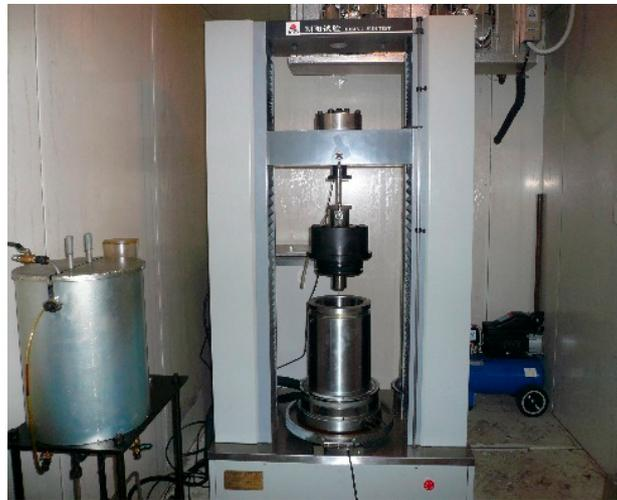
Figure 2. Appearance of the triaxial test system.
