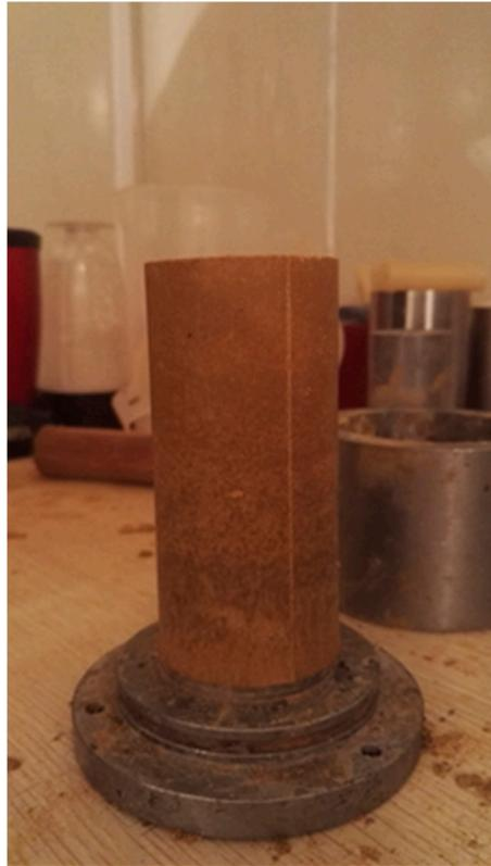
**Figure 6.** Samples of CH<sub>4</sub> hydrate-bearing sediments.
