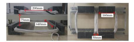
Figure 11. Setup of the transmitter coil and the receiver coils.
